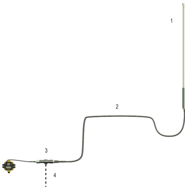
1. Antenna mounted remotely from the radio device.
