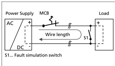
Maximal wire length for a magnetic (fast) tripping \*):
