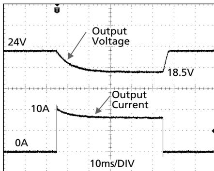
Peak load 10A (resistive load) for 50ms
