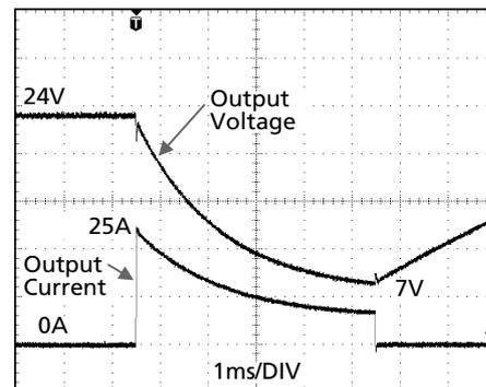
Peak load 25A (resistive load) for 5ms
