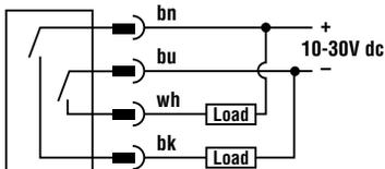
NOTES: Output Type for all models is Bipolar NPN/PNP. Load 150 mA max., each output.
