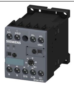
SOLID-STATE TIME-DELAY RELAY MULTI-FUNCTION, 16 FUNCTIONS 2 CHANGEOVER CONTACTS AC/DC 24 TO 240V 0.05 S TO 100H WIDTH 45MM SCREW TERMINALS
