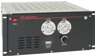
**5U Series** — Rack Mounted, Adjustable Outputs of 0.5 – 15 psig OR 0.5 – 30 psig. The 5U series is our most popular Rack Mounted dehydrator. With its higher flow capability of the 1/4hp compressor, it's ideally suited for systems with multiple waveguides. The extra flow also helps compensate for systems that experience high leak rates due to aging gaskets and seals. Just like our 3U series, the 5U can be offered with OPM and ERM monitoring options.
