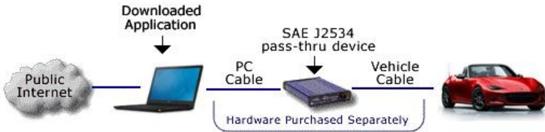
Hardware validated by Mazda can be purchased separately from a third-party supplier. Validation has been done using the following J2534 pass-thru device and cables:
