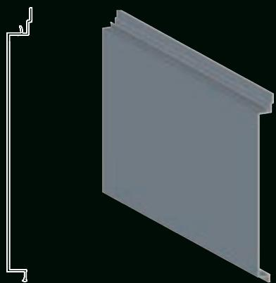
Alucovering® 01/C Horizontal Butt Joint
