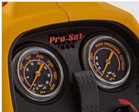
High and low pressure gauges
