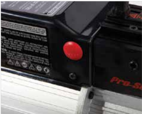
Manual reset button HP switch (TR21E only)
