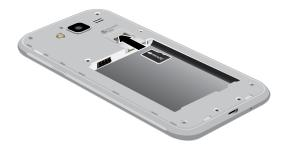
Slide the memory card into the slot with the gold contacts facing down.
