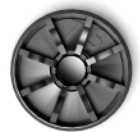
Plastic Support after Hammering (8 supporting block become deformed, and fit with the screw)
