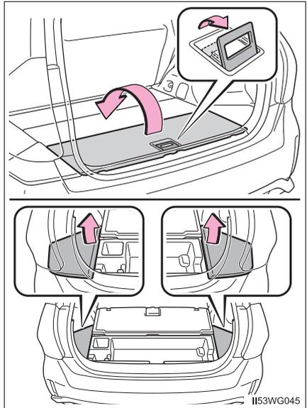
Lift the center deck board and then lift the side deck boards.
