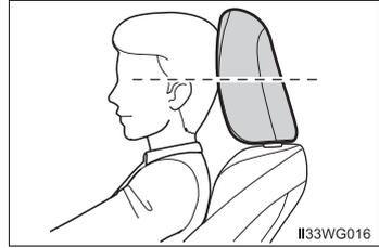
**■ Adjusting the center rear seat head restraint**
