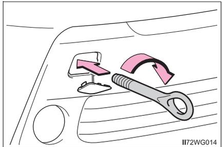
4 Tighten down the towing eyelet securely using a wheel nut wrench or hard metal bar.
