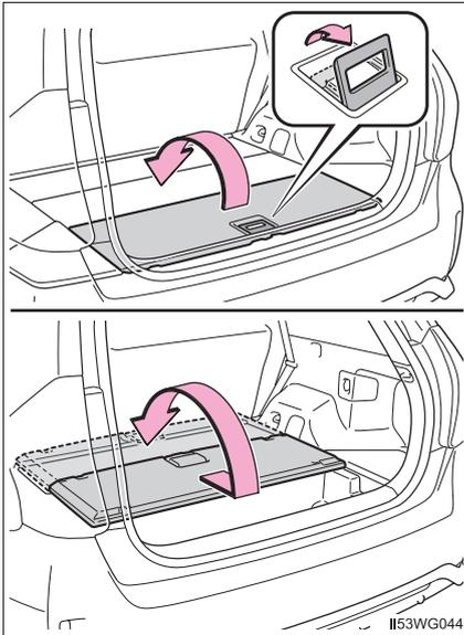
Pull the lever upward to lift the deck board.
