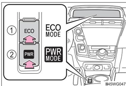
When the “ECO” switch is pressed, the “ECO MODE” indicator comes on in the instrument cluster.
