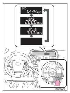
Switches between odometer and trip meter displays. When the trip meter is displayed, pressing and holding the "TRIP" button will reset the trip meter.
