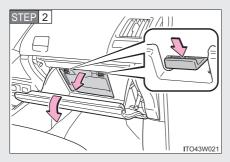
Open the glove box and remove the filter exchange cover.
