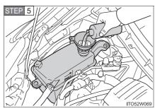
If necessary, add engine coolant up to the "FULL" line.
