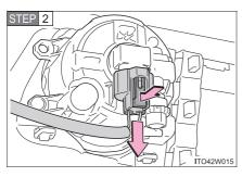
Unplug the connector while pressing the lock release.
