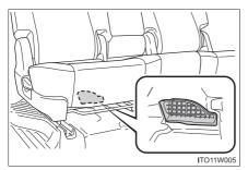
There is an air intake vent under the rear seat for the purpose of cooling the hybrid battery (traction battery). If the vent becomes blocked, the hybrid battery (traction battery) may overheat, leading to a reduction in hybrid battery (traction battery) output.
