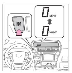
Press the button to switch the display between MPH and km/h.
