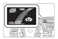
Hybrid System Indicator represents the hybrid system power output and regenerative charging. (→P. 203)
