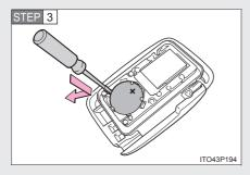
Remove the depleted battery.
