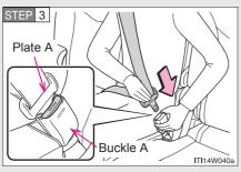
Secure the belt by inserting plate A into buckle A until a click sound is heard.
