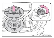
Unload the tool holder from the vehicle and loosen the center fastener that secures the spare tire.
