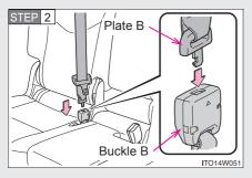
Connect by inserting plate B into buckle B until a click sound is heard.
