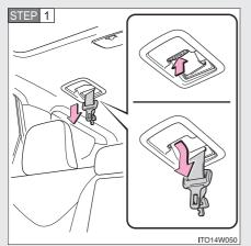
Press the plate to release, and pull out the seat belt.
