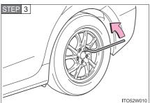
Slightly loosen the wheel nuts (one turn).
