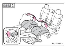
Pull the seatback angle adjustment lever to flatten the seatback.
