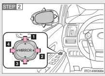
To adjust the mirror, press the switch.
