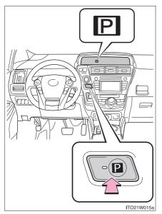
Fully stop the vehicle and set the parking brake, and then press the P position switch.
