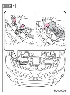
For the right side only: Remove the bolt and unclip the engine coolant reservoir hose. Then lift up the air cleaner inlet duct.
