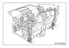
The pretensioner helps the seat belt to quickly restrain the occupant by retracting the seat belt when the vehicle is subjected to certain types of severe frontal or side collision.
