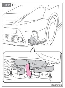
Remove the engine under cover bolts and pull down the engine under cover.
