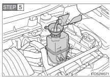
If necessary, add power control unit coolant up to the "F" line.
