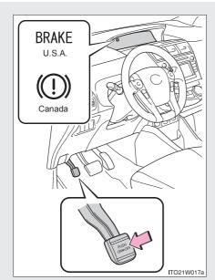
To set the parking brake, fully depress the parking brake pedal with your left foot while depressing the brake pedal with your right foot.
