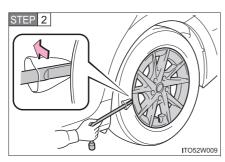
For vehicles with 16 inch wheels, remove the wheel ornament using the wrench.
