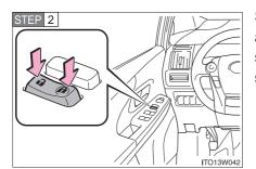
Shift the shift position to P or N, and press and hold the door lock switch ( or or o) for about 5 seconds then release.
