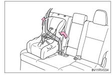
6 If the child restraint has a top tether strap, the top tether strap should be latched onto the top tether strap anchor. (→P. 69)
