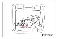
3 Push the lever for the back door motor.
