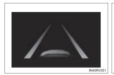
Indicates that the system is recognizing white (yellow) lines. When the vehicle departs from its lane, the white line displayed on the side the vehicle departs from flashes amber.
