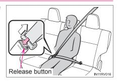
2 To release the hooked plate "A", insert the plate "B" or mechanical key (→P. 104) into the hole on the buckle.
