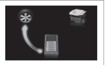
When the vehicle is powered by both the gasoline engine and the electric motor (traction motor)
