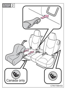
Latch the hooks of the lower straps onto the LATCH anchors.
