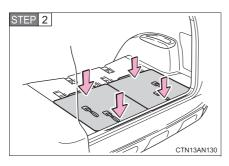
Push the seat on the front side against the floor and push the seat on rear side against the floor.
