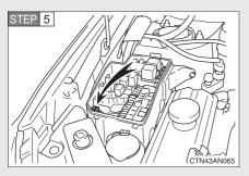
Remove the fuse with the pullout tool.
