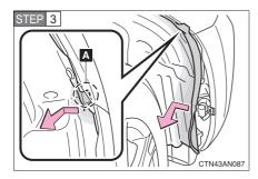
Move section "A" of the fender liner to the inner side of the vehicle, partly removing it and thereby allowing access to the front fog light.
