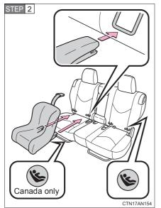
Latch the buckles onto the LATCH anchors.
