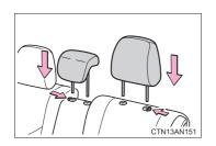
Align the head restraint with the installation holes and push it down while pressing the lock release button.
