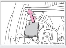
Type B: Push the tab in and lift the lid off.
