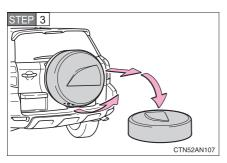
Remove the spare tire cover by holding the bottom and lifting it up and away from the vehicle.
