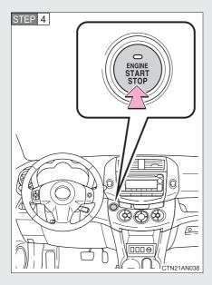
Press the "ENGINE START STOP" switch.
