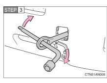
Tighten down the towing eyelet securely using a wheel nut wrench.
