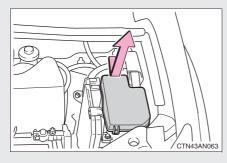
Type A: Push the tab in and lift the lid off.
