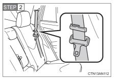
Make sure the outside seat belt passes through the hanger when folding the second seat.
