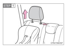
Remove the head restraint.
