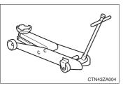
Lift up the vehicle using a floor jack such as the one shown in the illustration
