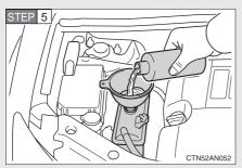
Add engine coolant if necessary.
