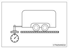
The load placed on the trailer hitch ball. ( $\rightarrow$ P. 230)
