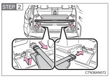
Insert the right end of the luggage cover into the recess, then compress the left end of the luggage cover and insert it into the recess.
