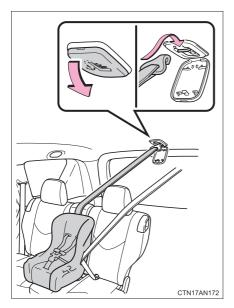
Open the anchor bracket cover. Secure the child restraint using the seat belt. Latch the hook onto the anchor bracket and tighten the top tether strap.
