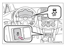
Push and hold the switch while the vehicle is stopped to turn off TRAC and VSC.
