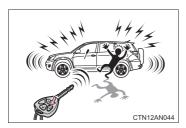
When **(t)** is pushed for longer than about one second, an alarm will sound for about 60 seconds and the vehicle lights will flash to deter any person from trying to break into or damage your vehicle.
