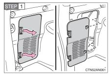
Disengage the claws and remove the cover.
