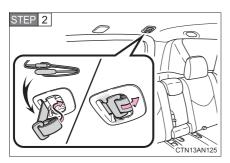
Stow the seat belt tabs in the cover located on the roof as shown.
