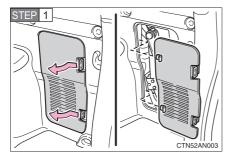
Disengage the claws and remove the cover.
