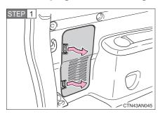
Open the back door  $(\rightarrow P. 48)$  and remove the cover.
