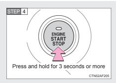
Vehicles with a smart key system: Stop the engine by pressing and holding the "ENGINE START STOP" switch for 3 consecutive seconds or more.
