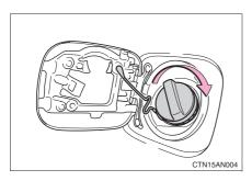
When replacing the fuel tank cap, turn it until a clicking sound is heard.
