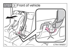
Secure the child restraint using the seat belt. Latch the hook onto the anchor bracket and tighten the top tether strap.
