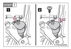
Right side only: Remove the clip and move it aside to allow easy access to the light bulbs.
