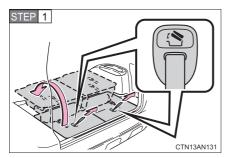
Pull the seat lock release strap, lift the seat up and move the seat forward. Lock the seat into place.
