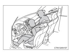
The pretensioner helps the seat belt to quickly restrain the occupant by retracting the seat belt when the vehicle is subjected to certain types of severe frontal collision or a vehicle rollover.
