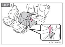
Pull the seatback angle adjustment lever up to unlock and push down the seatback.
