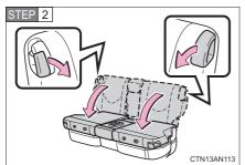
Pull down the seatback angle adjustment lever and fold down the seatback.
