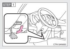
Hold the steering wheel and press the lever down.
