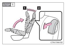
Fold the seatback while pulling the lever. Return the seatback and secure it at the 1st lock position (most upright position). Adjust the seatback to the 7th lock position.  $(\rightarrow P. 57)$
