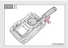
Remove the depleted battery.
