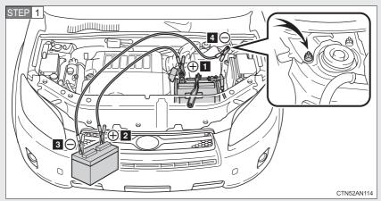
Connecting the jumper cables
