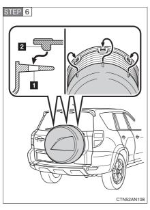
Insert the hooks into the upper slots and lower the cover to install the spare tire cover.
