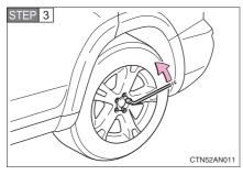
Slightly loosen the wheel nuts (one turn).
