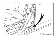
For the GAWR, see the Certification Label. For the maximum load of the tire, see the load limit at maximum cold tire inflation pressure mentioned on the sidewall of the tire. ( $\rightarrow$ P. 517)
