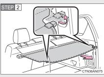
Pull out the luggage cover and hook onto the anchors.
