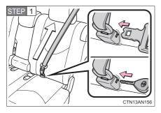
To release the tab "A", insert the tab "B", key (vehicles without a smart key system) or mechanical key (vehicles with a smart key system) ( $\rightarrow$ P. 26) into the hole on the buckle.
