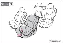
Slide the front seat further forward than the front-most lock position.
