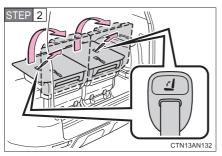
Pull the seatback lock release strap and raise the seatback.
