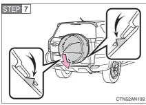
Attach the cover by hooking the 2 inner protrusions.
