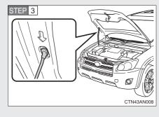
Hold the hood open by inserting the supporting rod into the slot.
