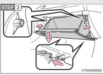
Push in each side of the glove box to disconnect the claws.
