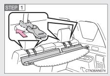
Attach the hooks to the head restraints.
