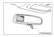
STEP 1 Push and hold the "AUTO" button for 6 to 12 seconds.
