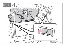
Open the back door and pull the lock release lever to fold down the second seat.
