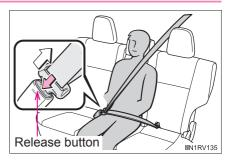
2 To release the hooked plate "A", insert the mechanical key (→P. 96) or plate "B" or the wireless key into the hole on the buckle.
