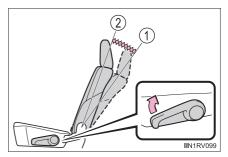
If your child restraint system interferes with a head restraint and cannot be installed properly, install the child restraint system after removing the head restraint. (→P. 147)
