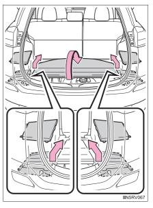
2 Insert the right end of the rear cargo net into the recess, then compress the left end of the rear cargo net and insert it into the recess.
