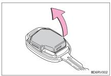
3 Open the case cover using a coin protected with tape etc. and remove the depleted battery.
