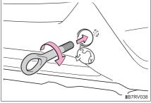
3 Tighten down the towing eyelet securely using a wheel nut wrench.
