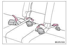
3 Lower the head restraint to the lowest position. ( $\rightarrow$ P. 147)
