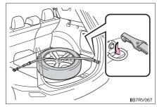
5 Pull the belt as shown in the illustration to secure the tire.
