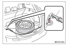
3 Pass the belts from between the wheel spokes through the center hole.
