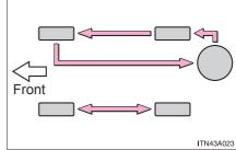
Do not fail to initialize the tire pressure warning system after tire rotation. To equalize tire wear and extend tire life, Toyota recommends that tire rotation is carried out at the same interval as tire inspection.
