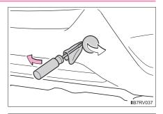
2 Insert the towing eyelet into the hole and tighten partially by hand.
