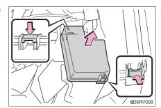
▶ Under the instrument panel Remove the cover.
