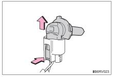
4 Replace the light bulb, and install the bulb base.
