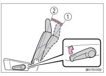
If your child restraint system interferes with a head restraint and cannot be installed properly, install the child restraint system after removing the head restraint. ( $\rightarrow$ P. 147)
