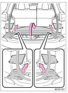
2 Insert the right end of the luggage cover into the recess, then compress the left end of the luggage cover and insert it into the recess.
