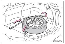
4 Hook one end of the forked belt to the cargo hook on the far right side, and the other end to the cargo hook on the near left side.
