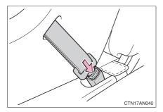
Push the buckle release button and fully retract the seat belt.
