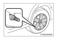
Align the cutout of the wheel ornament with the valve stem as shown.
