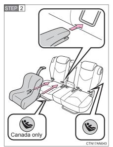
Latch the buckles onto the LATCH anchors.
