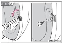
Remove the clip using a flathead screwdriver wrapped in a rag.
