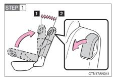
Fold the seatback while pulling the lever. Return the seatback and secure it at the 1st lock position (most upright position). Adjust the seatback to the 3rd lock position. ( $\rightarrow$ P. 54)
