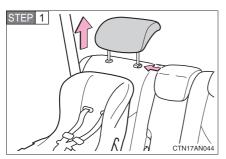
Remove the head restraint.
