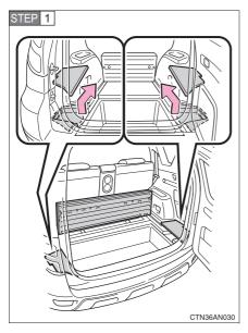
Open the rear deck board and remove the deck side cover.
