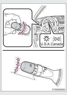
The side marker, parking, tail, license plate and instrument panel lights turn on.
