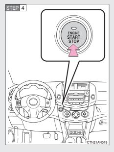
Press the "ENGINE START STOP" switch.
