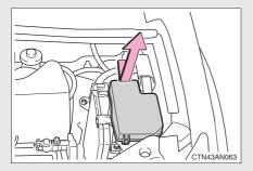
Type A: Push the tab in and lift the lid off.
