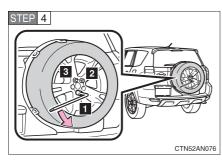
Using the wheel nut wrench, loosen the hold-down nuts by turning them counterclockwise until they can be loosened by hand. Follow the order shown in the illustration.
