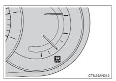
If the vehicle is in danger of slipping or if spins, the slip indicator light flashes to indicate that the Enhanced VSC/TRAC systems are operating.
