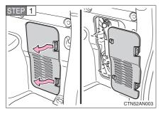
Disengage the claws and remove the cover.
