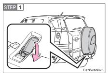
Open the back door. Unlock the latch handle which on the bottom of the spare tire cover.
