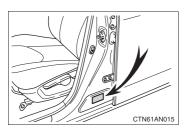
For the GAWR, see the Certification Label. For the maximum load of the tire, see the load limit at maximum cold tire inflation pressure mentioned on the sidewall of the tire.  $(\rightarrow P. 480)$
