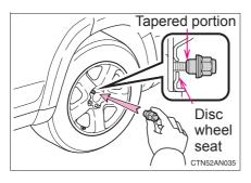
Tighten the nuts until the tapered portion comes into loose contact with the disc wheel seat.
