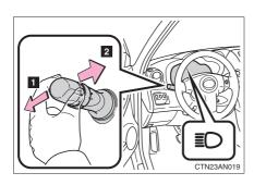
■ With the headlights on, push the lever forward to turn on the high beams.
