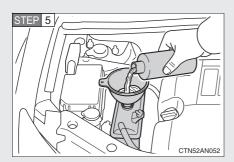
Add engine coolant if necessary.
