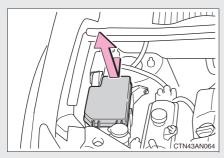
Type B: Push the tab in and lift the lid off.
