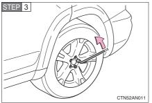
Slightly loosen the wheel nuts (one turn).
