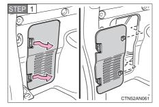
Disengage the claws and remove the cover.
