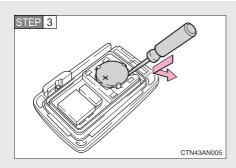
Remove the depleted battery.
