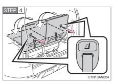
Pull the seatback lock release strap to fold down the seatback.
