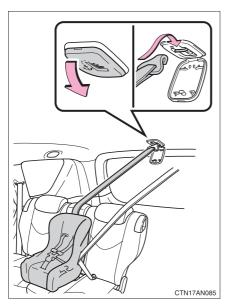
Open the anchor bracket cover. Secure the child restraint using the seat belt. Latch the hook onto the anchor bracket and tighten the top tether strap.
