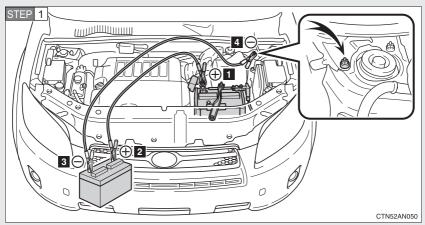
Connecting the jumper cables
