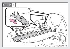
Attach the hooks to the head restraints.
