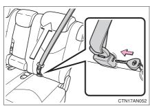
Second center seat: Release the center seat belt as shown in the illustration after removing the child restraint.
