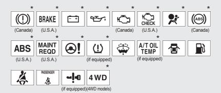
\*: These lights turn on when the "ENGINE START STOP" switch is turned to IGNITION ON mode (vehicles with smart key system) or the engine switch is turned to the "ON" position (vehicles without smart key system) to indicate that a system check is being performed. They will turn off after the engine is started, or after a few seconds. There may be a malfunction in a system if a light does not come on, or if the lights do not turn off. Have the vehicle inspected by your Toyota dealer for details.
