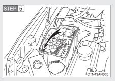
Remove the fuse with the pullout tool.
