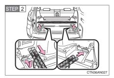
Insert the right end of the pipe into the recess, then compress the left end of the pipe and insert it into the recess.
