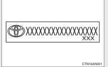
These labels are attached to the vehicle to reduce vehicle theft by facilitating the tracing and recovery of parts from stolen vehicles. Do not remove under penalty of law.
