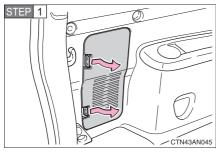
Open the back door  $(\rightarrow P. 46)$  and remove the cover.
