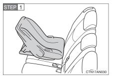
Place the child seat on the rear seat facing the rear of the vehicle.
