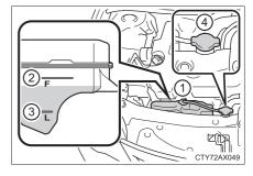
5 Add engine coolant if necessary.
