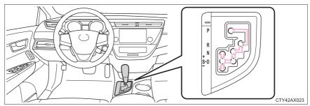
While the engine switch is in IGNITION ON mode, move the shift lever with the brake pedal depressed.
