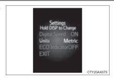
5 Press and hold the "DISP" button after selecting the "EXIT" by pressing the "DISP" button.
