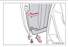
8 Reinstall the fender liner clips.
