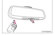
Test the operation of the HomeLink<sup>®</sup> by pressing the newly programmed button.
