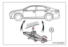
A Raise the vehicle until the tire is slightly raised off the ground.
