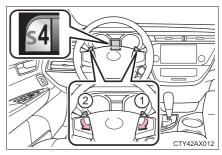
The initial shift range in S mode is set automatically to "4" or "5" according to vehicle speed. However, the initial shift range may be set to "3" if Al-SHIFT has operated while the shift lever was in the D position. ( $\rightarrow$ P. 168)
