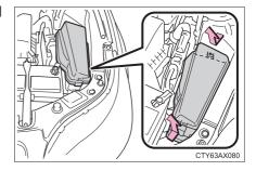
Driver's side instrument panel Remove the lid.
