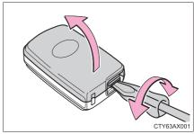
Remove the depleted battery.
