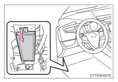
4 Remove the fuse with the pullout tool.
