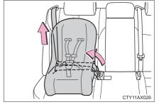
If the child restraint has a top tether strap, the top tether strap should be latched onto the top tether strap anchor.  $(\rightarrow P. 62)$
