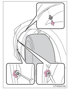
Remove the fender liner bolt and partly remove the fender liner.
