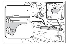
5 Add engine coolant if necessary.
