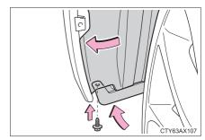
8 Reinstall the fender liner clips.
