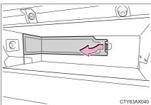
4 Press the tabs and remove the filter cover.
