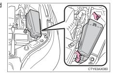
Driver's side instrument panel Remove the lid.
