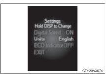
4 Press and hold the "DISP" button to select the desired setting.
