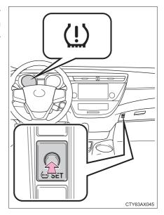
Wait for a few minutes with the engine switch in IGNITION ON mode and then turn the engine switch off.
