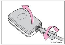
Remove the depleted battery.
