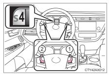
The initial shift range in S mode is set automatically to "4" or "5" according to vehicle speed. However, the initial shift range may be set to "3" if Al-SHIFT has operated while the shift lever was in the D position. ( $\rightarrow$ P. 164)
