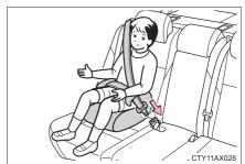
Check that the shoulder belt is correctly positioned over the child's shoulder and that the lap belt is as low as possible.
