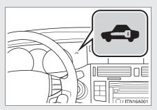
The indicator light flashes after the "ENGINE START STOP" switch or the engine switch has been turned off to indicate that the system is operating.
