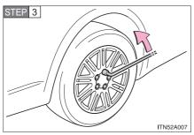
Slightly loosen the wheel nuts (one turn).
