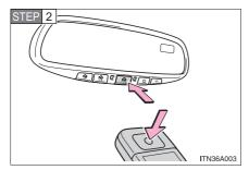
Press and hold down one of the buttons on the HomeLink<sup>®</sup> and the button on the transmitter. Continue holding down both buttons until the HomeLink<sup>®</sup> indicator light changes from a slow blink to a rapid flash. This will take approximately 30 seconds.
