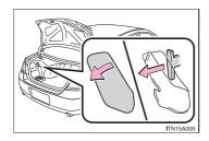
The lever can be used to open the fuel filler door if the fuel filler door cannot be opened using the inside switch because the battery discharged or for any other reason.
