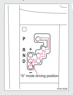
While the "ENGINE START STOP" switch or the engine switch is in ON mode, depress the brake pedal and move the shift lever.
