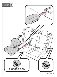
Latch the buckles onto the anchorages.
