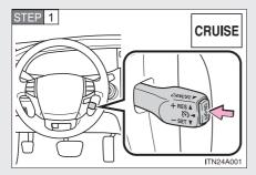
Press the "ON-OFF" button to operate the cruise control.
