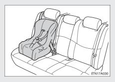
Seat belts equipped with a child restraint locking mechanism (ALR/ELR belts except driver's seat belt) (→P. 56)
