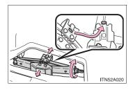
To store the jack, align the hole of the jack head with the vehicle hook. Turn the jack joint until the jack base fits securely with the vehicle body.
