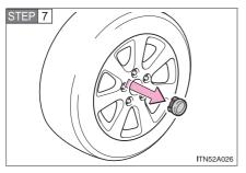
Type B: Remove the wheel ornament by pushing from the reverse side.
