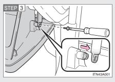
Open the glove box. Remove the screw with a Phillips-head screwdriver and slide off the damper.
