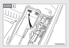
Remove the fuse with the pullout tool.
