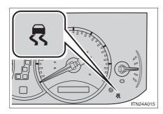
If the vehicle is in danger of slipping, or if the front wheels spin, the slip indicator light flashes to indicate that the VSC/TRAC have been engaged.
