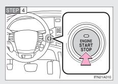
Press the "ENGINE START STOP" switch.
