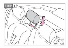
Secure the child restraint using a seat belt or lower anchors, and lock the head restraint in place at the lowest position.
