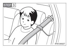
Buckle, position and release the seat belt.
