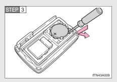
Remove the depleted battery.
