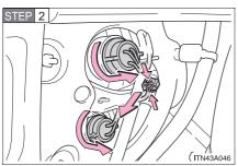
Turn the bulb bases counterclockwise and remove (upper and lower), or squeeze bulb base and remove (center).
