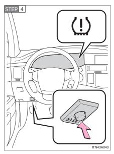
Push and hold the tire pressure warning reset switch until the tire pressure warning light blinks slowly three times.
