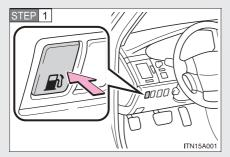
Press the fuel filler door opener switch.
