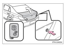
Press the button to unlock the trunk.
