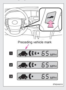
Each push of the switch changes the vehicle-to-vehicle distance
