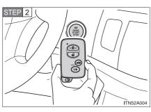
Touch the Toyota emblem side of the electronic key to the "ENGINE START STOP" switch.
