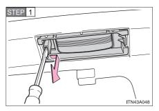
Use a flathead screwdriver to disengage the side of the lamp.
