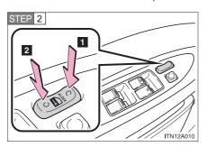
Shift the shift lever to "P" or "N", press and hold the driver's door lock switch (1 or 2) for about 5 seconds then release.
