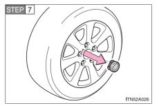
Type B: Remove the wheel ornament by pushing from the reverse side.
