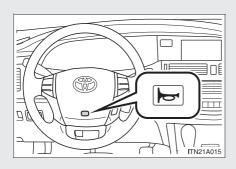
To sound the horn, press on or close to the key mark.
