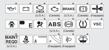
\*:These lights turn on when the "ENGINE START STOP" switch is turned to IGNITION ON mode (vehicles with smart key system) or the engine switch is turned to the "ON" position (vehicles without smart key system) to indicate that a system check is being performed. They will turn off after the engine is started, or after a few seconds. There may be a malfunction in a system if the lights do not come on, or turn off. Have the vehicle inspected by your Toyota dealer.
