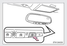
Press the button for longer than 3 seconds to turn auto mode on/off.
