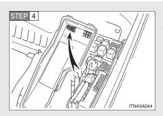
Remove the fuse with the pullout tool.
