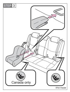
Latch the buckles onto the LATCH anchors.
