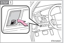
Press the fuel filler door opener switch.
