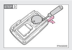
Remove the depleted battery.
