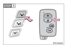
Push the "1" or "2" button on the driver's side and the button on the wireless remote control at the same time for about 1 second until you hear a beep.
