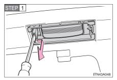
Use a flathead screwdriver to disengage the side of the lamp.
