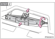
To remove the jack, turn the jack joint by hand until the jack becomes free.
