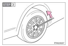
Slightly loosen the wheel nuts (one turn).
