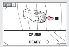
Press the "ON-OFF" button to operate the cruise control.
