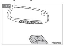
Point the remote control for the device 1 to 3 in. (25 to 75 mm) from the HomeLink® control buttons as shown in the illustration.
