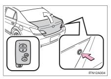
Press the button to unlock the trunk.
