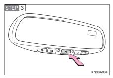
Test the HomeLink<sup>®</sup> operation by pressing and holding the newly programmed button for 2 seconds. If programming was successful, the garage door will open and close.
