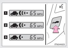
Each push of the switch changes the vehicle-to-vehicle distance
