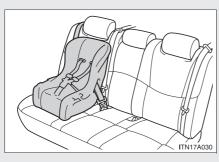
Seat belts equipped with a child restraint locking mechanism (ALR/ELR belts except driver's seat belt) (→P. 59)
