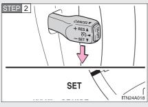
Accelerate or decelerate to the desired speed and press the lever down to set the cruise control speed.
