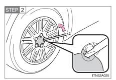
Type A: Remove the wheel ornament using the wheel nut wrench.
