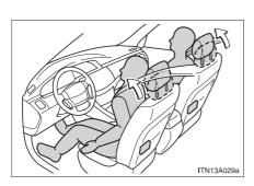
When a front seatback receives a strong impact during a rearend collision, the head restraint moves slightly forward and upward to provide support for the occupants head.
