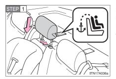
Secure the child restraint using a seat belt or LATCH anchors, and lock the head restraint in place at the lowest position.
