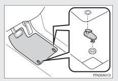
Secure the floor mat using the hooks provided.
