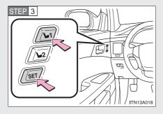
Push the "SET" button, then within 3 seconds, push button "1" or "2" until the signal beeps.
