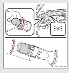
The side marker, parking, tail, license plate and instrument panel lights turn on.
