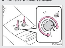
Press the knob to turn the system on, and turn the knob to the desired temperature setting.
