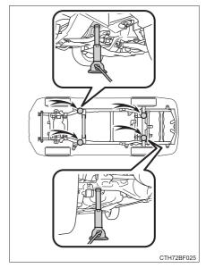
Raise the vehicle until the tire is slightly raised off the ground.
