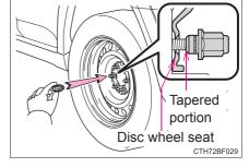
When replacing an aluminum wheel with an aluminum wheel, tighten the wheel nuts until the washers comes into contact with the disc wheel.
