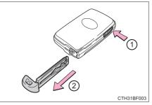
After using the mechanical key, store it in the electronic key. Carry the mechanical key together with the electronic key. If the electronic key battery is depleted or the entry function does not operate properly, you will need the mechanical key.  $(\rightarrow P. 450)$
