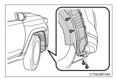
3 Partly remove the fender liner.
