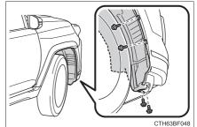
3 Partly remove the fender liner.
