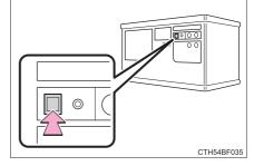
3 Press and hold the programmed HomeLink® button (located inside the vehicle) for 2 seconds and release it. Repeat this sequence (press/hold/release) up to 3 times to complete programming.
