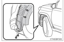
3 Partly remove the fender liner.
