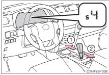
The initial shift range in S mode is set automatically to "4" according to vehicle speed. However, the initial shift range may be set to "3" if Al-SHIFT has operated while the shift lever was in the D position.  $(\rightarrow P. 202)$
