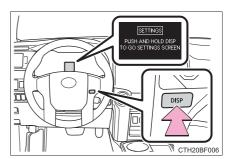
Press the "DISP" switch to select the item to be set, then press and hold the "DISP" switch.
