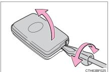
Remove the depleted battery.
