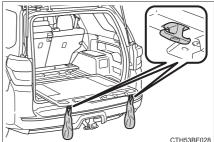
Type B only: To use the grocery bag hooks, slide the slide deck to the full-slide locked position.  $(\rightarrow P. 308)$
