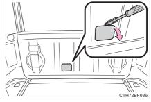
2 Tear the plastic film. Remove the cover.
