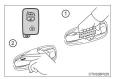
2 Touch the lock sensor (the indentation on the upper part of the door handle) to lock the doors.
