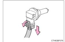
Replace the light bulb, and install the bulb base.
