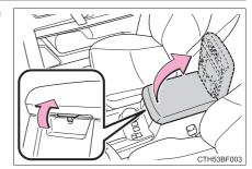
■The separator can be used in either of the positions shown in the illustration
