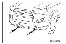
Vehicles with front covers only: Before using the front emergency towing eyelet(s), remove the cover(s).
