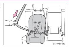
4 While pushing the child restraint system into the rear seat, allow the shoulder belt to retract until the child restraint system is securely in place.
