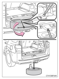
3 Pull out the spare tire and remove the holding bracket.
