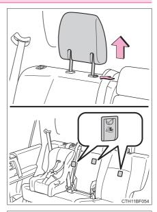
Open the anchor bracket cover, latch the hook onto the anchor bracket and tighten the top tether strap.
