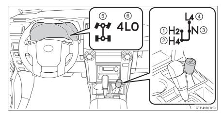
The four-wheel drive indicator comes on when H4, N or L4 mode is selected.
