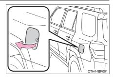
2 Turn the fuel tank cap slowly to open. Hang the fuel tank cap on the back of the fuel filler door.
