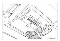
2 Press and hold one of the HomeLink® buttons and the transmitter button. When the HomeLink® indicator light changes from a slow to a rapid flash, you can release both buttons.
