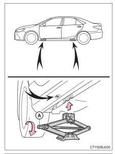
Raise the vehicle until the tire is slightly raised off the ground.
