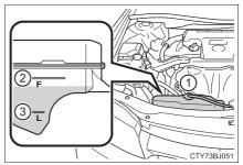
Power control unit coolant reservoir
