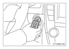
3 Firmly depress the brake pedal and check that 🚉 is displayed on the multi-information display.
