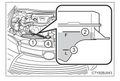
5 Add engine coolant if necessary.
