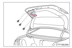
2 Unplug the connector while depressing the lock release.
