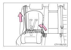
5 If the child restraint has a top tether strap, the top tether strap should be latched onto the top tether strap anchor. (→P. 65)
