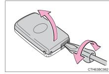
Remove the depleted battery.
