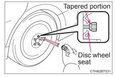
When replacing an aluminum wheel with a steel wheel, tighten the wheel nuts until the tapered portion comes into loose contact with the disc wheel seat.
