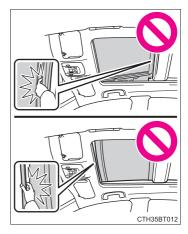
When exiting the vehicle, turn the engine switch off, carry the key and exit the vehicle along with the child. There may be accidental operation, due to mischief, etc., that may possibly lead to an accident.
