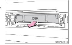
5 Remove the air conditioning filter from the filter case and replace it with a new one.
