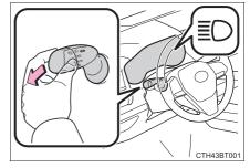
2 Press the Automatic High Beam switch.
