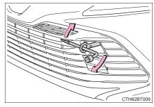
Securely attach cables or chains to the towing eyelet. Take care not to damage the vehicle body.
