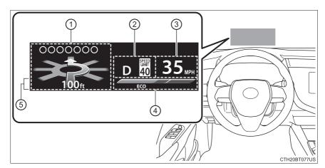
Driving assist system status/navigation system-linked display area (if equipped) (→P. 115)
