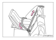
5 After installing the child restraint system, rock it back and forth to ensure that it is installed securely. (→P. 64)
