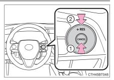
2 Pressing the "+ RES" switch resumes the cruise control and returns vehicle speed to the set speed.
