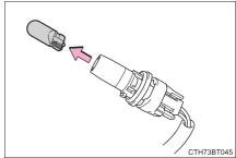
7 Install a new light bulb and then install the bulb base to the light unit by inserting it and turning it clockwise.
