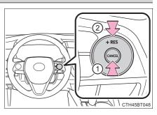
However, cruise control does not resume when the vehicle speed is approximately 25 mph (40 km/h) or less.
