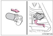
Connect the connector.(When replacing right side bulb only.)
