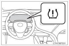
8 Vehicles with a tire inflation pressure display function: Drive straight (with occasional left and right turns) at approximately 25 mph (40 km/h) or more for approximately 10 to 30 minutes.
