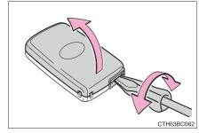
Remove the depleted battery.
