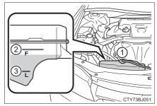
Power control unit coolant reservoir
