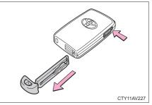
After using the mechanical key, store it in the electronic key. Carry the mechanical key together with the electronic key. If the electronic key battery is depleted or the entry function does not operate properly, you will need the mechanical key. ( $\rightarrow$ P. 485)
