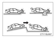
The SRS curtain shield airbags may also deploy under the situations shown in the illustration.
