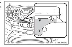
5 Add engine coolant if necessary.
