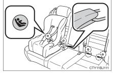
Seat belts equipped with a child restraint locking mechanism (ALR/ELR belts except driver's seat belt) (→P. 32)
