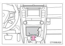
Open the cover and connect an iPod using an iPod cable. Turn on the power of the iPod if
