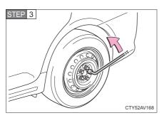
Slightly loosen the wheel nuts (one turn).
