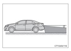
When any part of the vehicle sags due to the number of passengers or the distribution of the load, there is a margin of error between the fixed guide lines on the screen and the actual distance/course on the road.
