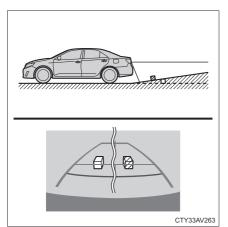
The distance guide lines will appear to be closer to the vehicle than the actual distance. Because of this, objects will appear to be farther away than they actually are. In the same way, there will be a margin of error between the guidelines and the actual distance/course on the road.
