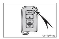
Press at twice while pressing and holding at . Confirm that the electronic key indicator flashes 4 times.
