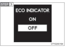
Press the "DISP" button to select the desired setting, and then press and hold the "DISP" button
