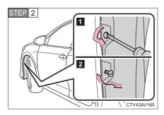
Remove the fender liner clip.
