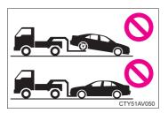
Be sure to transport the vehicle with the front wheels raised or with all four wheels raised off the ground. If the vehicle is towed with the front wheels contacting the ground, the drivetrain and related parts may be damaged or electricity generated by the operation of the motor may cause a fire to occur depending on the nature of the damage or malfunction.
