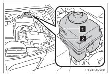
The brake fluid level should be between the "MAX" and "MIN" lines on the tank.
