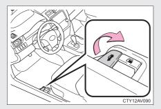
Pull up the lever to release the trunk lid.
