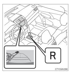
The rear view image is displayed when the shift position is in R and the "POWER" switch is in ON mode.
