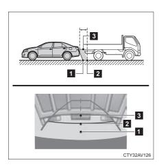
Visually check the surroundings and the area behind the vehicle. On the screen, it appears that a truck is parked at point 2. However, in reality if you back up to point 1, you will hit the truck. On the screen, it appears that 1 is closest and 3 is furthest away. However, in reality, the distance to 1 and 3 is the same, and 2 is farther than 1 and 3.
