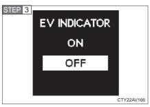
Press the "DISP" button to select the desired setting, and then press and hold the "DISP" button.
