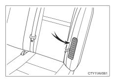
There is an air intake vent beside the rear left seat for the purpose of cooling the hybrid battery (traction battery). If the vent becomes blocked, the hybrid battery may overheat, leading to a reduction in hybrid battery output.
