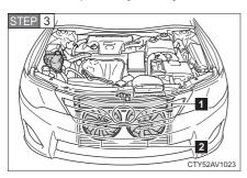
After the hybrid system has cooled down, inspect the hoses and radiator core (radiator) for any leaks.
