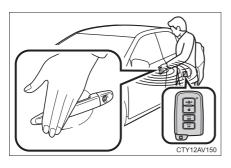
Touch the lock sensor (the indentation on the side of the door handle) to lock the doors.
