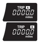
Displays the distance the vehicle has been driven since the meter was last reset. Trip meters A and B can be used to record and display different distances independently.
