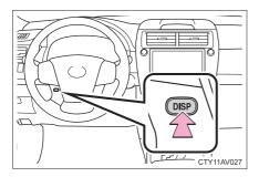
Push the "DISP" switch on the steering wheel several times to select the energy monitor display. (→P. 185)
