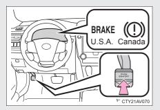
To set the parking brake, fully depress the parking brake pedal with your left foot while depressing the brake pedal with your right foot.
