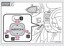
To adjust the mirror, press the switch.
