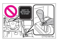
Check that the shift lever is securely set in P. The hybrid system may not start if the shift lever is displaced out of P. "SHIFT TO P POSITION TO START" will be displayed on the multi-information display.
