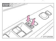
Shift the shift lever to P or N, and press and hold the driver's door lock switch ( or or ) for approximately 5 seconds and then release.
