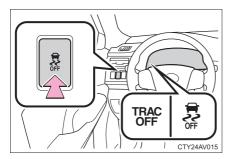
Push and hold the switch for more than 3 seconds while the vehicle is stopped to turn off TRAC and VSC.
