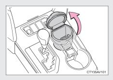
An ashtray can be installed in the cup holder. ( $\rightarrow$ P. 372)
