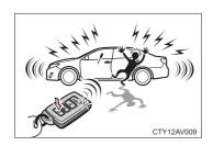
When ((t) is pressed for longer than about one second, an alarm will sound intermittently and the vehicle lights will flash to deter any person from trying to break into or damage your vehicle.
