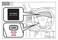
Press the "DISP" button to display the setting screen while the vehicle is stopped, and then press and hold the "DISP" button to display the customize mode screen.
