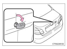
Turn the mechanical key clockwise to open.
