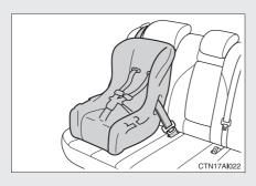
Seat belts equipped with a child restraint locking mechanism (ALR/ELR belts except driver's seat belt) (→P. 57)
