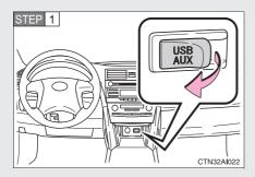
Open the cover and connect an iPod<sup>®</sup> using an iPod<sup>®</sup> cable.
