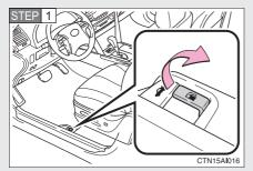
Pull the lever to open the fuel filler door.
