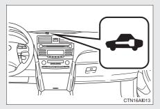
Vehicles with smart key system: The indicator light flashes after the "ENGINE START STOP" switch has been turned OFF to indicate that the system is operating.
