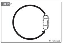
Drive the vehicle at 5 mph (8 km/h) or less in a circle until a direction is displayed.
