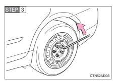
Slightly loosen the wheel nuts (one turn).
