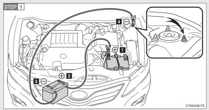
Connecting the jumper cables
