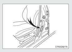
One of the following labels will be attached to the driver's side center pillar.
