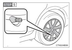
For vehicles with a steel wheel, reinstall the wheel ornament.
