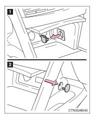
The auxiliary box of the front console is provided with a hole that allows cables to be passed into the cabin from the power outlet and AUX or USB/AUX adapter inside.
