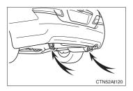
When your vehicle becomes stuck and cannot move, the emergency hooks are used for another vehicle to pull your vehicle out in an emergency.
