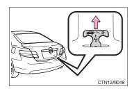
The trunk lid can be opened by pulling up the glow-in-the-dark lever located on the inside of trunk lid.
