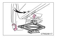
The jack point guides are located under the rocker panel. They indicate the jack point positions.
