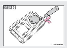
Remove the depleted battery.
