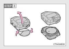
Open the case cover using a coin protected with tape etc. and remove the depleted battery.
