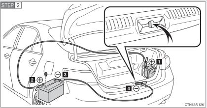
Connecting the jumper cables
