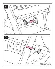
The auxiliary box of the front console is provided with a hole that allows cables to be passed into the cabin from the inside power outlet and AUX or USB/AUX adapter.
