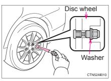
Turn the nut washers until they come into contact with the disc wheel.
