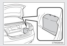
The 12-volt battery is located in the right-hand side of the luggage compartment.
