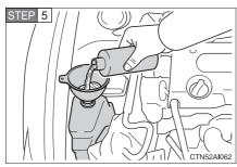
Add engine coolant if necessary.
