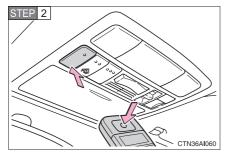
Press and hold down one of the buttons on HomeLink® and the button on the transmitter. When the indicator light on HomeLink® changes from a slow to a rapid flash after 20 seconds, you can release both buttons.
