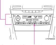
Rear window defogger switch/ Rear window defogger switch and outside rear view mirror defogger switch \* P. 188
