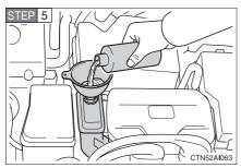
Add power control unit coolant if necessary.
