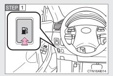
Press the fuel filler door opener switch.
