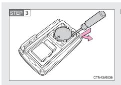
Remove the depleted battery.
