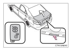
Press the button to unlock the trunk.
