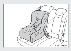
Seat belts equipped with a child restraint locking mechanism (ALR/ELR belts except driver's seat belt) (→P. 62)
