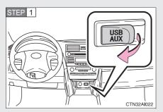
Open the cover and connect an iPod<sup>®</sup> player using an iPod<sup>®</sup> cable.
