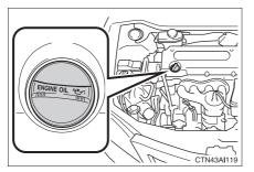
If the oil level is below or near the low level mark, add engine oil of the same type as already in the engine.
