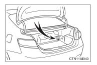
Never try to open the service plug access hole located in the luggage compartment. The service plug is used only when the vehicle is serviced and is subject to high voltage.
