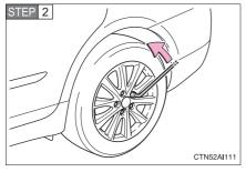
Slightly loosen the wheel nuts (one turn).
