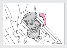
An ashtray can be installed in a cup holder. ( $\rightarrow$ P. 294)
