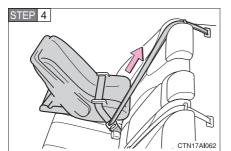
While pushing the child seat down into the rear seat, allow the shoulder belt to retract until the child seat is securely in place.
