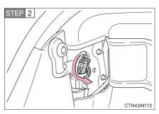
Turn the bulb bases counter-clockwise.
