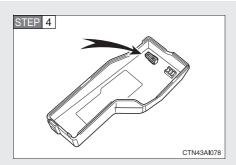
Remove the fuse with the pullout tool.
