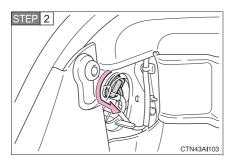
Turn the bulb bases counter-clockwise.
