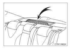
There is an air intake vent on the package tray for the purpose of cooling the hybrid battery (traction battery). If the vent becomes blocked, the hybrid battery may overheat, leading to a reduction in hybrid battery output.
