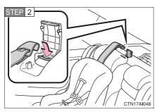
Open the anchor bracket cover, latch the hook onto the anchor bracket and tighten the top strap.
