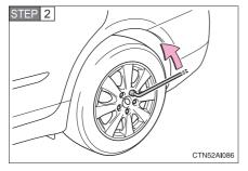
Slightly loosen the wheel nuts (one turn).
