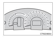
The brightness of the arcs around the fuel economy meter and speedometer change according to the eco drive level. The higher the fuel economy, the brighter the light becomes.
