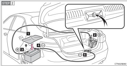
Connecting the jumper cables
