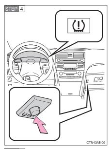
Open the glove box, and press and hold the tire pressure warning reset switch until the tire pressure warning light blinks slowly three times.
