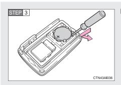
Remove the depleted battery.
