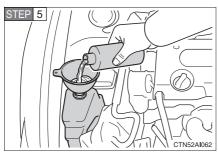
Add engine coolant if necessary.
