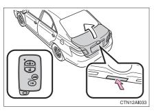
Press the button to unlock the trunk.
