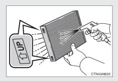
If the filter is dirty, clean by blowing compressed air through the filter from the bottom.
