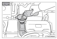
Add power control unit coolant if necessary.
