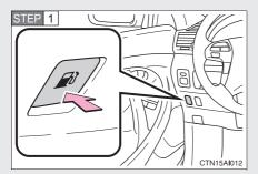
Press the fuel filler door opener switch.
