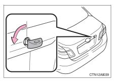
Turn the mechanical key counterclockwise to lock the trunk opener feature.
