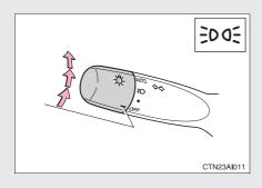
The side marker, parking, tail, license plate and instrument panel lights turn on.
