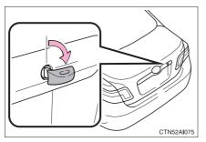
Turn the mechanical key clockwise to open.
