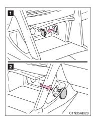
The auxiliary box of the front console is provided with a hole that allows cables to be passed into the cabin from the inside power outlet and AUX adapter.
