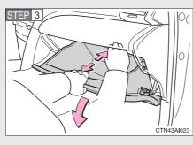
Apply pressure to the glove box as shown to disconnect the claws.
