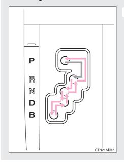
While the "POWER" switch is in ON mode, depress the brake pedal and move the shift lever.
