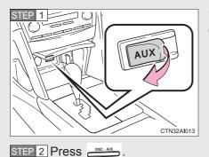
Connect the portable audio device.
