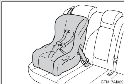
Seat belts equipped with a child restraint locking mechanism (ALR/ELR belts except driver's seat belt) (→P. 55)
