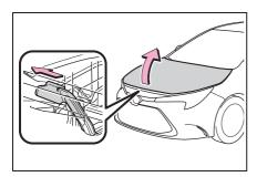
3 Hold the hood open by inserting the support rod into the slot.
