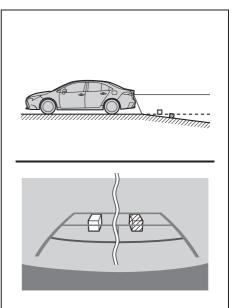
The distance guide lines will appear to be further from the vehicle than the actual distance. Because of this, objects will appear to be closer than they actually are. In the same way, there will be a margin of error between the guide lines and the actual distance/course on the road.
