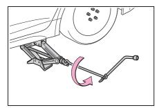
**4** Firmly tighten each wheel nut two or three times in the
