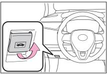
2 Pull the auxiliary catch lever to the left and lift the hood.
