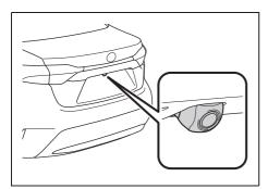
The camera for the rear view monitor system is located as
