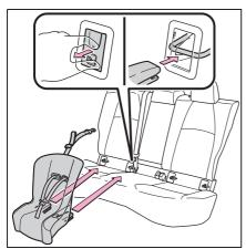
3 If the child restraint has a top strap, follow the child restraint manufacturer's operation manual regarding the installation, using the top strap to latch onto the top strap anchorage. (→P.68)
