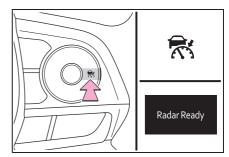
Accelerate or decelerate, with accelerator pedal operation, to the desired vehicle speed (at or above approximately 20 mph [30 km/h]) and press the "-SET" switch to set the speed.
