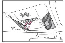
1 Turns the door position on/off When a door is opened while the door position is on, the lights turn on.
