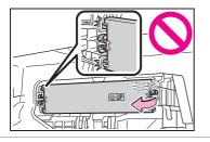
Cleaning the hybrid battery (traction battery) air intake vent and filter
