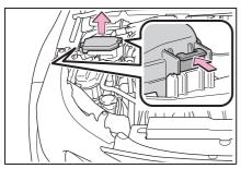
► Engine compartment: type B fuse box
