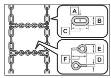
A Side chain (0.12 in. [3 mm] in diameter)
