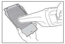
6 Reinstall the filter to the cover.
