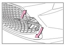
5 Securely attach cables or chains to the towing eyelet. Take care not to damage the vehicle body.
