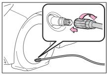
Make sure that the compressor switch is off.
