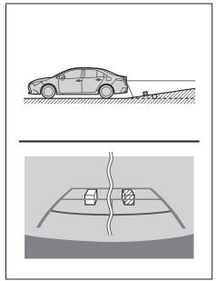
The distance guide lines will appear to be closer to the vehicle than the actual distance. Because of this, objects will appear to be farther away than they actually are. In the same way, there will be a margin of error between the guide lines and the actual distance/course on the road.
