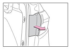
4 Remove the 2 screws and then remove the light assembly by pulling it straight back.
