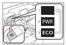
Each time the switch is pressed, the system changes between power mode, normal mode and Eco drive mode.
