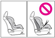
\*3: If the head restraint interferes with your child restraint system, and the head restraint can be removed, remove the head restraint.
