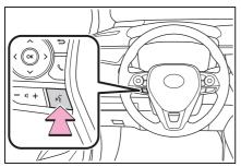
The voice command system and its list of commands can be operated. (→P.334)
