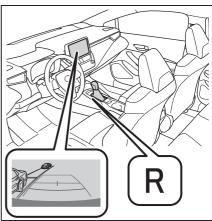
The rear view monitor system will be deactivated when the shift lever is shifted to any position other than R.
