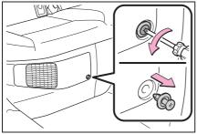
3 Remove the air intake vent cover.
