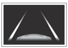
Indicates that the system is recognizing white (yellow) lines or a course\*. When the vehicle departs from its lane, the white line displayed on the side the vehicle departs from flashes orange.
