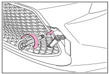
4 Tighten down the towing eyelet securely using a wheel nut wrench (if equipped) or hard metal bar.
