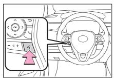
Voice guidance for the voice command system can be skipped by pressing the talk switch.
