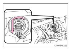
Pull the bulb out while pressing the lock release of the connector.
