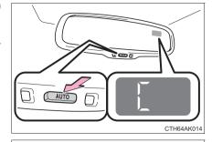
(8 km/h) or less in a circle until a direction is displayed. If there is not enough space to drive in a circle, drive around the block until the direction is displayed.
