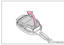
3 Open the case cover using a coin protected with tape etc. and remove the depleted battery using a small flathead screwdriver.
