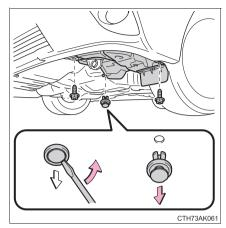
2 Partly remove the fender liner.
