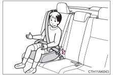
Check that the shoulder belt is correctly positioned over the child's shoulder and that the lap belt is as low as possible.  $(\rightarrow P. 28)$
