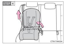
While pushing the child seat into the rear seat, allow the shoulder belt to retract until the child seat is securely in place.
