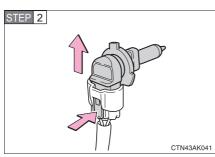
Unplug the bulb while depressing the lock release.
