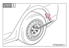
Slightly loosen the wheel nuts (one turn).
