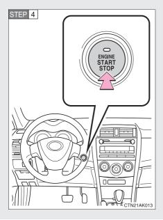
Press the "ENGINE START STOP" switch.
