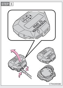
Open the case cover using a flathead screwdriver protected with tape etc. and remove the depleted battery.
