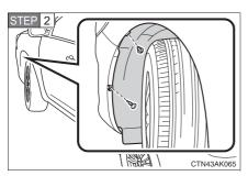
Remove the fender liner clips.
