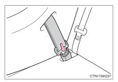
Push the release button and fully retract the seat belt.
