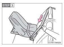
Fully extend the shoulder belt and then allow it to retract slightly in order to activate the ALR lock mode.
