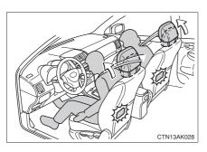
When a front seatback receives a strong impact, the head restraint moves slightly forward to help reduce the risk of whiplash on the seat occupant.
