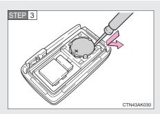
Remove the depleted battery.
