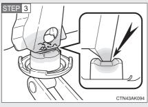
Before raising the vehicle, make sure that the floor jack is positioned so that the jack point fits securely inside the groove on the jack attachment.
