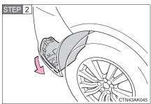
Partly remove the fender liner.
