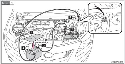
Connecting the jumper cables
