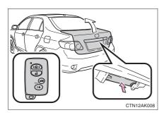
Press the button to unlock the trunk.
