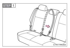
Rear right seat only: Slide the rear center seat belt to the side to prevent it from getting pinched in the lower anchorage.
