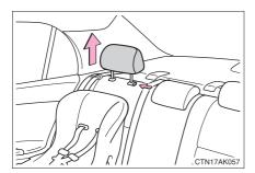
Remove the head restraint.
