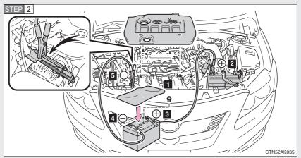
Connecting the jumper cables
