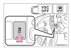
Push and hold the button while the vehicle is stopped to turn off TRAC and VSC.
