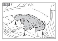
Remove the fender liner bolts and clip.
