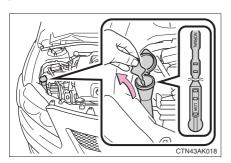
Check the washer fluid level on the level gauge. If the washer fluid level is at "LOW", add washer fluid.
