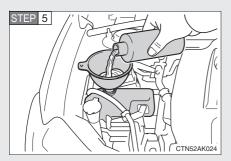
Add engine coolant if necessary.
