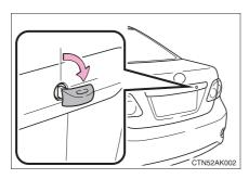
Turn the mechanical key clockwise to open.
