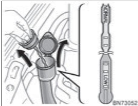
**For vehicles sold in the U.S.A.**—If any washer does not work, the washer tank may be empty. Check the washer fluid level on the level gauge. If the washer fluid level is at “LOW”, add washer fluid.
