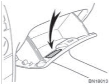
The air conditioning filter information label is placed inside of the glove box as shown and indicates that a filter has been installed.
