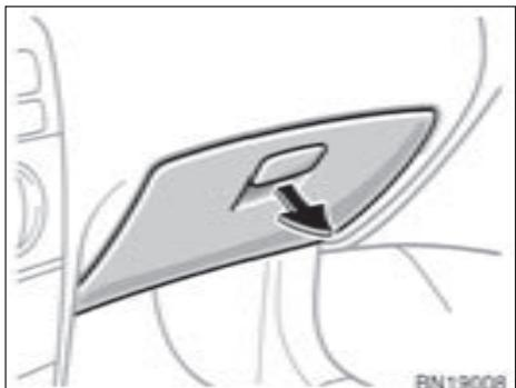
To open the glove box door, pull the lever.
