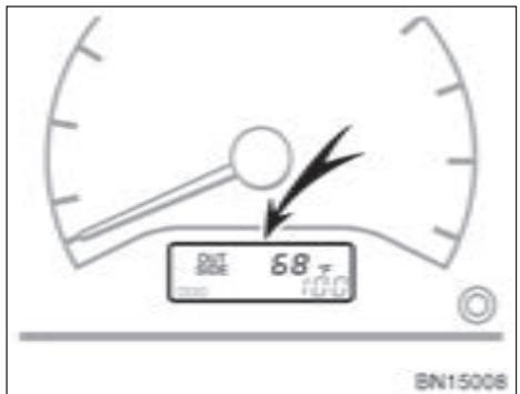
The displayed temperature ranges from  $-30^{\circ}\text{C}$  ( $-22^{\circ}\text{F}$ ) up to  $50^{\circ}\text{C}$  ( $122^{\circ}\text{F}$ ).
