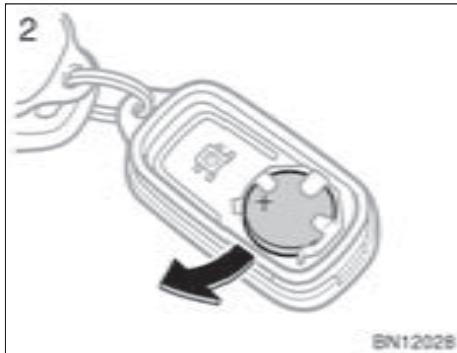
2. Remove the discharged transmitter battery.
