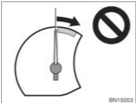
The tachometer indicates engine speed in thousands of rpm (revolutions per minute). Use it while driving to select correct shift points and to prevent engine luggering and over-revving.
