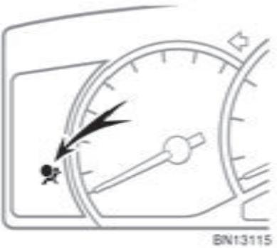
**This indicator comes on when the ignition key is turned to the “ON” position. It goes off after about 6 seconds. This means the SRS front airbags are operating properly.**
