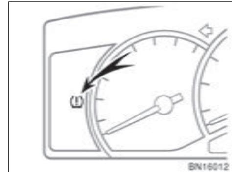
The tire pressure warning light comes on when the ignition key is turned to the “ON” position and goes off after a few seconds. This means the tire pressure warning system is operating properly. If the tire inflation pressure becomes low, the light comes on again. In this case, adjusting the tire inflation pressure will turn off the light after a few minutes. If the light comes on after blinking for 1 minute, the tire pressure warning system is not working properly.
