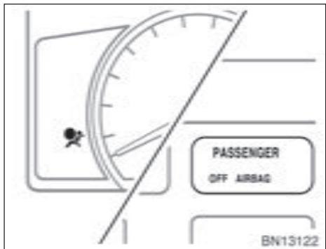
The SRS warning light will come on and front passenger occupant classification indicator light will indicate "OFF" if there is a malfunction in the front passenger occupant classification system.
