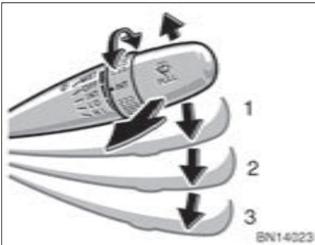
**To turn on the windshield wipers, move the lever to the desired setting.**
