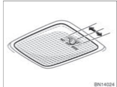
To turn on the interior light, slide the switch.
