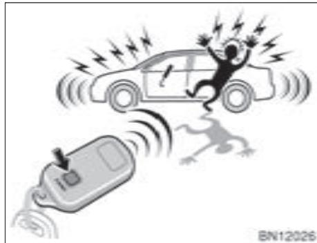
**Pushing the “PANIC” switch blows the horn intermittently and flashes the headlights, tail lights, turn signal lights and interior light.**
