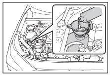
6 Start the hybrid system and turn the air conditioning system on to check that the radiator cooling fan operates and to check for coolant leaks from the radiator or hoses.
