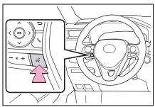
The voice command system and its list of commands can be operated. (→P.470)
