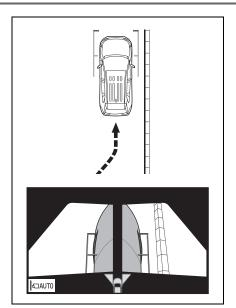
Pull over to the curb as shown in the illustration above, taking care not to let the vehicle width guide line overlap the target object.
