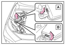
► Engine compartment: Type B fuse box
