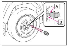
When replacing an aluminum wheel with an aluminum wheel, turn the wheel nuts until the washers (|A|) come into contact with the disc
