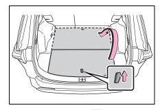
Place the edge A into the groove, and with the deck board in a standing state, put the edge B into the holes.
