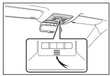
It is unnecessary to speak directly into the microphone when giving a command.
