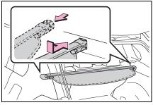
Pull out the luggage cover and hook it onto the anchors.
