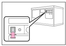
3 Press and hold the desired HomeLink® button (inside the vehicle) for 2 seconds and release it. Repeat this sequence (press/hold/release) up to 3 times to complete programming. If the garage door opener motor operates when the HomeLink® button is pressed, the garage door opener motor recognizes the HomeLink® signal.
