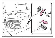
3 Remove the air intake vent cover.
