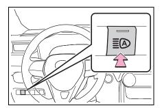
2 Push the lever away from you with the headlight switch in the △UTO or ■○ position.
