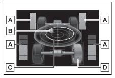
A Torque distribution display Displays the drive status of each wheel in 6 steps from 0 to 5.
