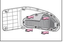
7 Install the air intake vent cover.
