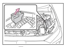
4 Connect a positive jumper cable clamp to A on your vehicle and connect the clamp on the other end of the positive cable to B on the second vehicle. Then, connect a negative cable clamp to C
