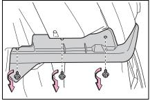
**3** Remove the screws and clips, partly remove the fender liner.
