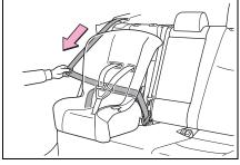
6 While pushing the child restraint system into the rear seat, allow the shoulder belt to retract until the child restraint system is securely in place.
