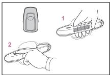
1 Grip the driver's door handle to unlock the door. Holding the driver's door handle for approximately 2 seconds unlocks all the doors. Grip the front passenger's door handle or rear door handle (some models) to unlock all the doors\*.
