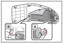
Engage the 4 center claws to install the filter.
