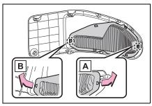
**5** Remove the dust and clogs from the filter using a vacuum cleaner, etc.
