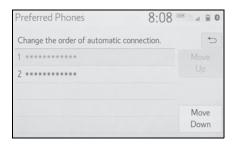
A newly registered Bluetooth<sup>®</sup> device will automatically be given the highest automatic connection priority.
