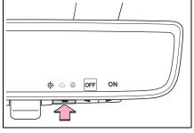
3 Press or to enable (ON)/disable (OFF) the automatic anti-glare function.
