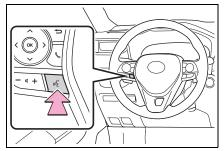
The voice command system and its list of commands can be operated. (→P.470)
