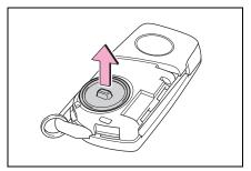
**3** Remove the depleted battery.
