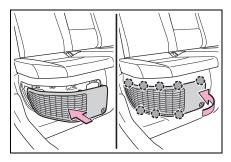
**8** Using a Phillips screwdriver, install the clip.
