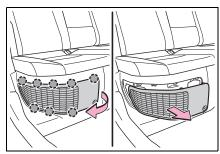
4 Remove the air intake vent filter.
