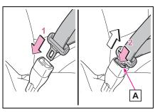
To fasten the seat belt, push the plate into the buckle until
