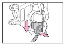
**5** Turn the bulb base counter-clockwise.
