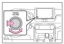
"POWER VOLUME" knob: Press to turn the audio/visual system on and off. The system turns on in the last mode used. Turn this knob to adjust the volume.
