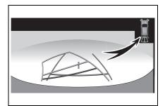
A simplified image is displayed on the upper corner of the screen when an obstacle is detected.
