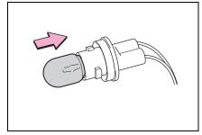
Install the bulb base to the light unit by inserting it and turning the bulb base clockwise.
