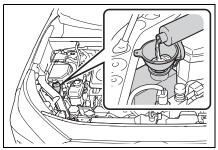
6 Start the hybrid system and turn the air conditioning system on to check that the radiator cooling fan operates and to check for coolant leaks from the radiator or hoses.
