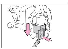
**5** Turn the bulb base counter-clockwise.
