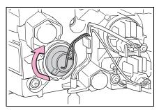
6 Align the grooves on the light unit with the claws, and insert the light unit straight so that the pin on the light unit fit into the hole.
