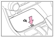
2 Place the charging side of the portable device down.
