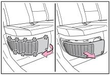
4 Remove the air intake vent filter.
