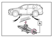
**4** Assemble the jack handle and the wheel nut wrench as shown in the illustration.
