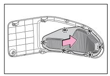
7 Install the air intake vent cover.
