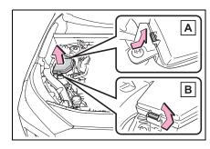
▶ Engine compartment: Type B fuse box
