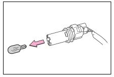
3 Install a new light bulb then install the bulb base to the light unit by inserting it and turning the bulb base clockwise.
