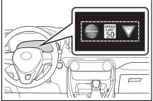
When a tab other than the driving support system information display is selected, only a recognized speed limit sign or do not enter sign (when notification is necessary) will be displayed.
