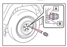
When replacing an aluminum wheel with an aluminum wheel, turn the wheel nuts until the washers (A) come into contact with the disc
