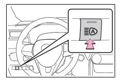
2 Push the lever away from you with the headlight switch in the △UTO or **SO** position.
