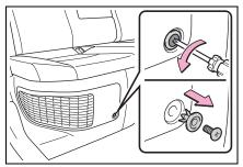
3 Remove the air intake vent cover.
