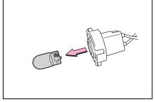
8 Install a new light bulb then install the bulb base to the light unit by inserting it and turning the bulb base clockwise.
