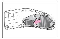
5 Remove the dust and clogs from the filter using a vacuum cleaner, etc.
