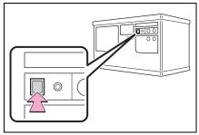
HomeLink® button (inside the vehicle) for 2 seconds and release it. Repeat this sequence (press/hold/release) up to 3 times to complete programming.
