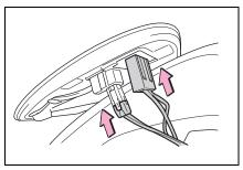
**13**Align the tabs, and secure the mirror by pushing in each diagonally-opposite pair of tabs in order.
