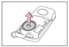
3 Remove the depleted battery.
