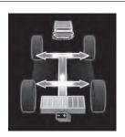
▶ When the vehicle is powered by both the gasoline engine and the electric motor (traction motor)
