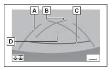
A Vehicle width guide line Displays a guide path when the vehicle is being backed straight up.
