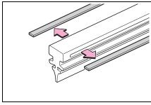
from the claw at the center of the wiper blade. Pass the wiper insert through the 3 claws so that it sticks out from the stopper, and then pass the wiper insert through the final remaining claw.
