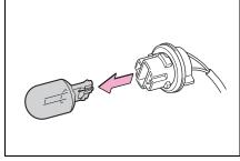
5 Install a new light bulb then install the bulb base to the light unit by inserting it and turning the bulb base clockwise.
