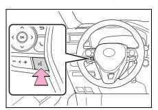
The voice command system and its list of commands can be operated. (→P.460)
