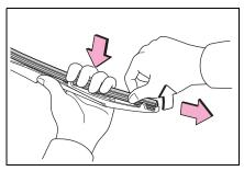
4 Remove the 2 metal plates from the old wiper insert and install them to the replacement wiper insert.
