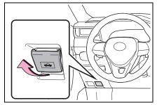
2 Push the auxiliary catch lever to the left and lift the hood.
