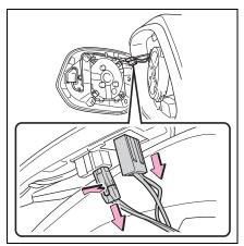
3 Disconnect the tabs behind the mirror cover, and remove the mirror cover.
