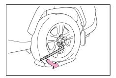
4 Turn the tire jack portion A by hand until the notch of the jack is in contact with the jack point.
