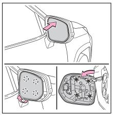
2 Disconnect the connectors behind the mirror, and remove the mirror.
