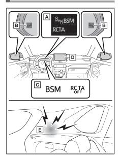
A Multi-information display Turning the BSM function/RCTA function on/off.
