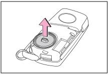
3 Remove the depleted battery.
