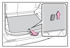
2 Place the deck board through the groove and move forward
