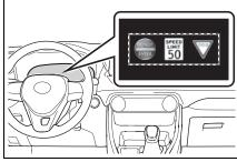
When a tab other than the driving support system information display is selected, only a recognized speed limit sign or do not enter sign (when notification is necessary) will be displayed. (→P.89)
