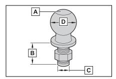
A Trailer ball load rating Matches or exceeds the gross trailer weight rating of the trailer.
