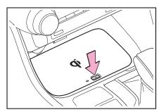
2 Place the charging side of the portable device down.
