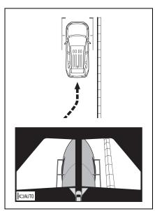
Pull over to the curb as shown in the illustration above, taking care not to let the vehicle width guide line overlap the target object.
