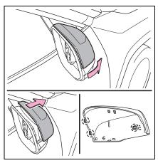
4 Fold the mirror before removing the light unit.
