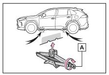
**5** Assemble the jack handle and the wheel nut wrench as shown in the illustration.
