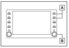
A Press to change the track. Press and hold to fast forward/rewind.
