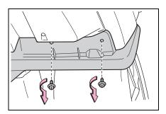
**3** Remove the screws and clips, partly remove the fender liner.
