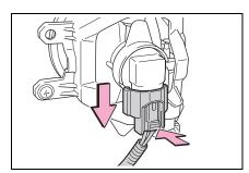
**5** Turn the bulb base counter-clockwise.
