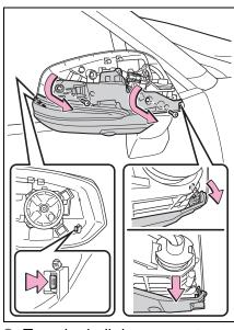
**6** Turn the bulb base counter-clockwise.
