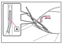
2 Lift the stopper using a flathead screwdriver as shown in the illustration.
