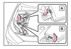
► Engine compartment: Type B fuse box
