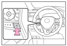
The voice command system and its list of commands can be operated. (→P.450)
