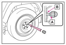
When replacing an aluminum wheel with a steel wheel, tighten the wheel nuts until the tapered portion
