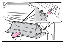
5 Unlock the filter cover (A), pull the filter cover out of the claws (B), and remove the filter cover.
