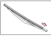
6 Check that the wiper blade claws are fitted in the grooves of the wiper insert.
