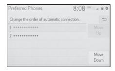
A newly registered Bluetooth<sup>®</sup> device will automatically be given the highest automatic connection priority.
