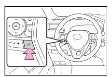
The voice command system and its list of commands can be operated. (→P.450)
