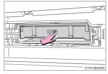
5 Remove the air conditioning filter from the filter case and replace it with a new one.
