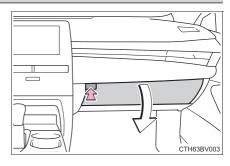
The glove box light turns on when the engine switch is in ACCESSORY or IGNITION ON mode.
