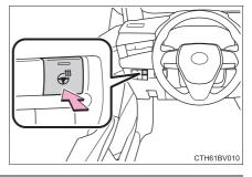
The heated steering wheel can be used when the engine switch is in IGNI-TION ON mode.
