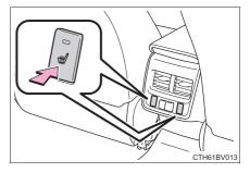
The seat heaters can be used when the engine switch is in IGNITION ON mode.
