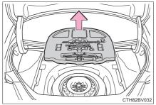
4 Loosen the center fastener that secures the spare tire.
