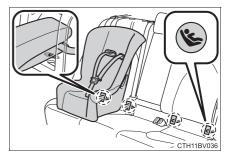
Seat belts equipped with a child restraint locking mechanism (ALR/ELR belts except driver's seat belt) (→P. 32)
