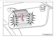
If the vanity lights remain on for 20 minutes while the engine is off, the lights will turn off automatically.
