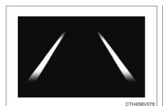
Indicates that the system is recognizing white (yellow) lines. When the vehicle departs from its lane, the white line displayed on the side the vehicle departs from flashes yellow.
