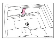
When the engine switch is turned off, the on/off state of the wireless charger will be memorized.
