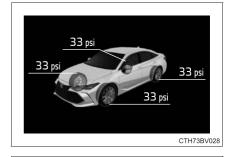
• If the tire pressure drops below a predetermined level, the driver is warned by a screen display and a warning light. (→P. 438)
