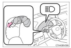
2 Press the Automatic High Beam switch.
