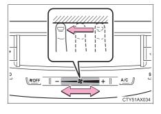
Touch \(\section{soft} to turn the fan off.
