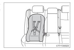
Run the seat belt through the child restraint system and insert the plate into the buckle. Make sure that the belt is not twisted.
