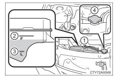
5 Add engine coolant if necessary.
