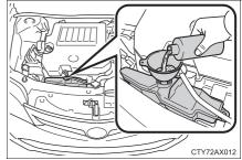
6 Start the engine and turn the air conditioning system on to check that the radiator cooling fans operate and to check for coolant leaks from the radiator or hoses.
