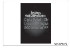
2 Press and hold the "DISP" button while the "Settings" screen is displayed.
