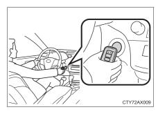
3 Firmly depress the brake pedal.
