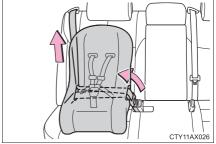
If the child restraint has a top tether strap, the top tether strap should be latched onto the top tether strap anchor.  $(\rightarrow P. 64)$
