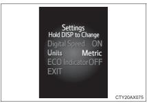
To exit the "Settings" screen, press the "DISP" button repeatedly until "EXIT" is highlighted and then press and hold the "DISP" button.
