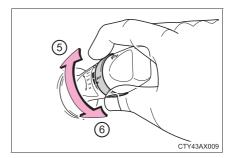
Wiper intervals can be adjusted for intermittent operation (when is selected).
