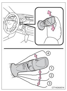
When "AUTO" is selected, the sensor sensitivity can be adjusted as follows by turning the switch ring.
