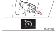
Accelerate or decelerate the vehicle to the desired speed, and push the lever down to set the speed.
