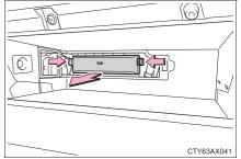
Remove the air conditioning filter and replace it with a new one.
