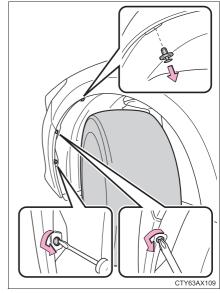
Remove the fender liner bolt and partly remove the fender liner.
