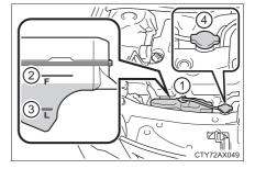
5 Add engine coolant if necessary.
