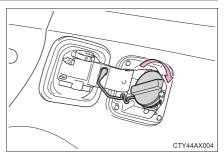
2 Close the fuel filler door, and press the center of the rear edge of the fuel filler door until you hear a click.
