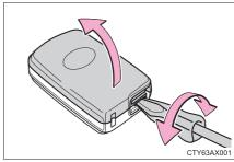
3 Remove the depleted battery.
