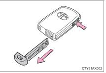
After using the mechanical key, store it in the electronic key. Carry the mechanical key together with the electronic key. If the electronic key battery is depleted or the entry function does not operate properly, you will need the mechanical key.  $(\rightarrow P. 411)$
