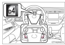
When a shift range higher than "5" is selected, the shift range will return to the normal D position.
