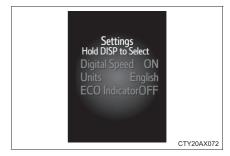
2 Press and hold the "DISP" button while the "Settings" screen is displayed.
