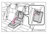
2 Pull the loop of wire to unlock the trunk lid.
