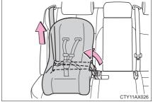
6 If the child restraint has a top tether strap, the top tether strap should be latched onto the top tether strap anchor. (→P. 64)
