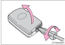
Remove the depleted battery.
