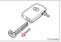
After using the mechanical key, store it in the electronic key. Carry the mechanical key together with the electronic key. If the electronic key battery is depleted or the entry function does not operate properly, you will need the mechanical key.  $(\rightarrow P. 410)$
