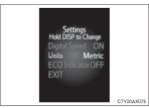
5 To exit the "Settings" screen, press the "DISP" button repeatedly until "EXIT" is highlighted and then press and hold the "DISP" button.
