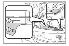
5 Add engine coolant if necessary.
