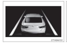
Indicates that the system is recognizing white (yellow) lines. When the vehicle departs from its lane, the white line displayed on the side the vehicle departs from flashes amber.
