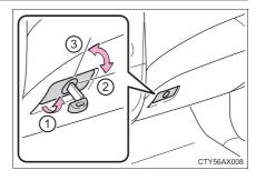
The trunk opener main switch is located in the glove box.  $(\rightarrow P. 104)$
