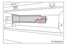
4 Press the tabs and remove the filter cover.
