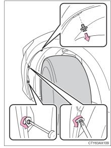
2 Remove the fender liner bolt and partly remove the fender liner.
