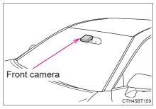
If the system judges that the vehicle is being driven over the speed limit, performing prohibited actions, etc. according to the recognized road signs, it notifies the driver through a visual notification and notification buzzer\*.
