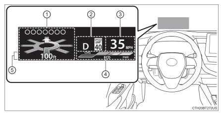
① Driving assist system status/navigation system-linked display area (if equipped) (→P. 140)
