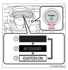
\*: If the shift lever is in a position other than P when turning off the hybrid system, the power switch will be turned to ACCESSORY mode, not to off.
