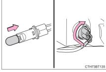
Align the tabs and push the light unit toward the front of the vehicle to install it.
