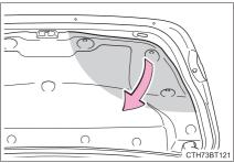
3 Disconnect the connector while depressing the lock release. (When replacing right side bulb only.)
