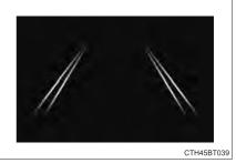
Indicates that the system is recognizing white (yellow) lines or a course\*. When the vehicle departs from its lane, the white line displayed on the side the vehicle departs from flashes yellow.
