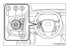
Pressing and holding the switch will display the first screen of the selected menu icon.
