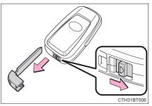
After using the mechanical key, store it in the electronic key. Carry the mechanical key together with the electronic key. If the electronic key battery is depleted or the entry function does not operate properly, you will need the mechanical key.  $(\rightarrow P. 539)$
