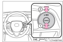
② Pressing the "+ RES" switch resumes the cruise control and returns vehicle speed to the set speed.
