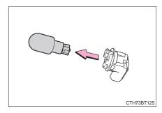
following Install a new light bulb and then install the bulb base to the light unit by inserting it and turning it clockwise.
