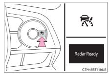
If the cruise control main switch is pressed and held for 1.5 seconds or more, the system turns on in constant speed control mode.  $(\rightarrow P. 306)$
