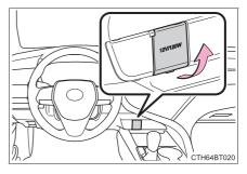
The power outlet can be used when the power switch is in ACCESSORY or ON mode.
