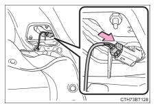
Reinstall the trunk lid cover with the clips.
