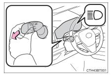
Press the Automatic High Beam switch.
