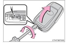
Remove the depleted battery using a small flathead screwdriver.
