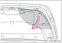
Jisconnect the connector while depressing the lock release. (When replacing right side bulb only.)
