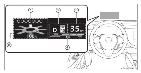
Driving assist system status/navigation system-linked display area (if equipped) (→P. 130)
