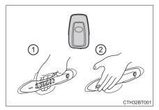
Make sure to touch the sensor on the back of the handle.
