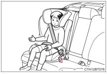
Check that the shoulder belt is correctly positioned over the child's shoulder and that the lap belt is as low as possible.  $(\rightarrow P. 28)$
