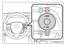
Large adjustment: Press and hold the switch to change the speed, and release when the desired speed is reached.
