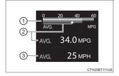
Displays the average vehicle speed since reset or elapsed time since reset, as selected in  $\bigcirc$  . ( $\rightarrow$ P. 105)
