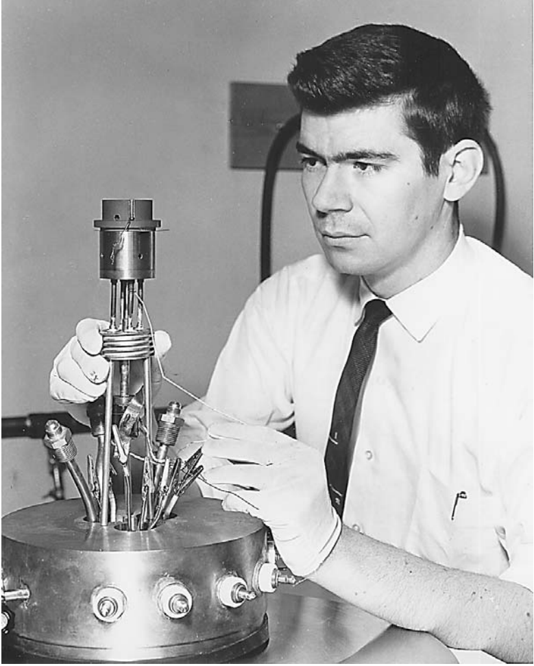
The young John Psarouthakis tests a thermo-ionic energy converter for space applications at MIT. Psarouthakis is a top-notch engineer.
