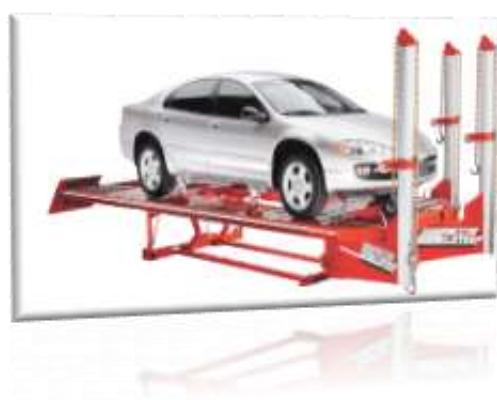
The course then progresses through frame damage and correction. Here we will introduce students to frame repair damage and directional pulls.
