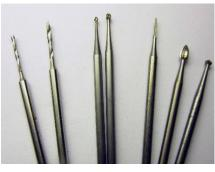
Ensure you have; Drills 0.7mm & 1.2mm. Setting burs 2.5mm & 3mm. Bud or cone bur 3mm. Hart bur 2.4mm
