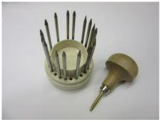
You will need a beading set to perform final claw tip shaping. A video is included showing how to other setting tools.
