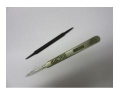
A scribe is a handy marking tool. I also recommend that you have a scalpel on hand for marking and removing bur flashing.
