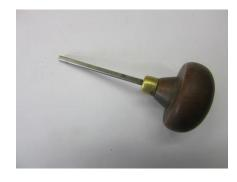
Claw tip shaping tool. This is something that is easy to make. It will help with closing the claw gap and final tip shaping.
