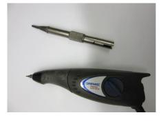
For claw setting hammer tools aren't essential. A hammer handpiece that fits to your pendant motor works well, but a Dremel tool is better.
