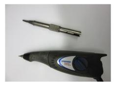
For finishing claw tips, using electric hammer tools aren't essential, but having this option can help to close stubborn gaps.
