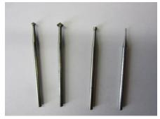
The recommended burs for this course are; Hart bur 1.2mm, 1.4mm, 1.6mm. Round bur 0.5 0.8mm, 1.7mm Cup bur 1.9mm. Tapered 1mm
