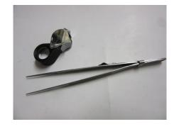
Stone tweezers and a jewellers loupe should always be close at hand. I also use an Optivisor with a 5x magnification lens.
