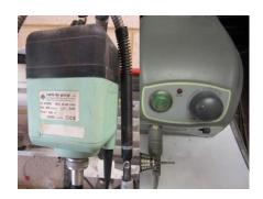
I generally use a micro motor for drilling & burring, but a standard pendant motor can be just as good if set up correctly.
