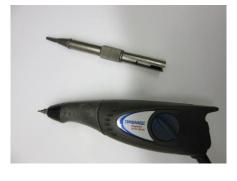
For bezel setting hammer tools will make the task easier. A hammer handpiece that fits to your pendant motor works well, but a Dremel tool is better.
