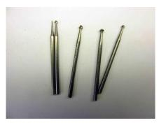
The recommended burs for this course are; Hart bur 1.5mm & 2mm & 3mm - 4mm. Round bur 0.5 mm 1.5mm & 1.8mm.
