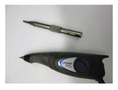
For a smooth bezel finish I recommend using electric hammer tools such as a Dremel with modified tips.
