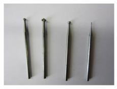
The recommended burs for this course are; Round bur 0.5mm, 0.8mm, 1.1mm, 1.7mm. Hart bur 1.2mm, 1.4mm, 1.6mm. Tapered 1mm
